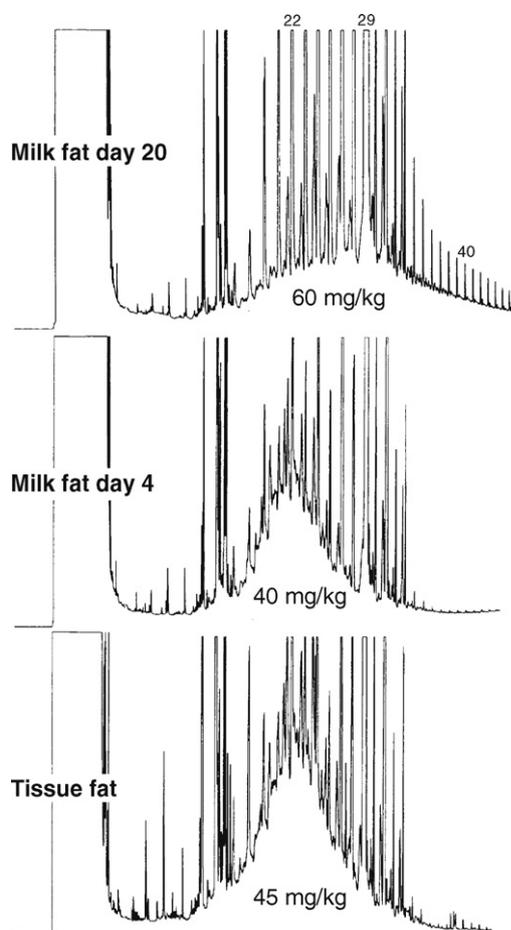
Fig. 6. Tissue and milk fat of day 4 showing the usual pattern of mineral paraffins. The milk fat of day 20, however, contained mineral paraffins at increased concentration and of a different composition. In this sample also most of the *n*-alkanes are of mineral origin as derived from the even-numbered species almost reaching the size of the odd-numbered.
