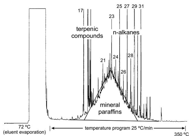
Fig. 1. Typical NPLC–NPLC–GC–FID chromatogram of a tissue fat. The mineral oil paraffins form the hump of unresolved components, the area of which is approximated by a triangle.
