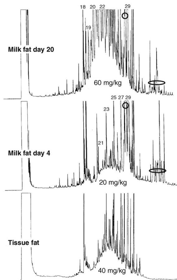
Fig. 7. Milk fats with non-identified hydrocarbons eluted in the region of the  $C_{40}$  alkanes (oval circles), a component eluted shortly before *n*- $C_{29}$  (round circles) and (day 20 milk) a complex mixture in the range of the  $C_{19}$ – $C_{25}$  *n*-alkanes.
